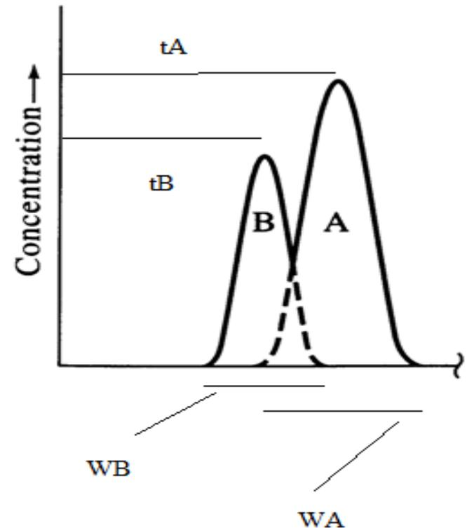
In case of mixing, we have to consider resolution factor  $R_s$  that can be determined by equation.
