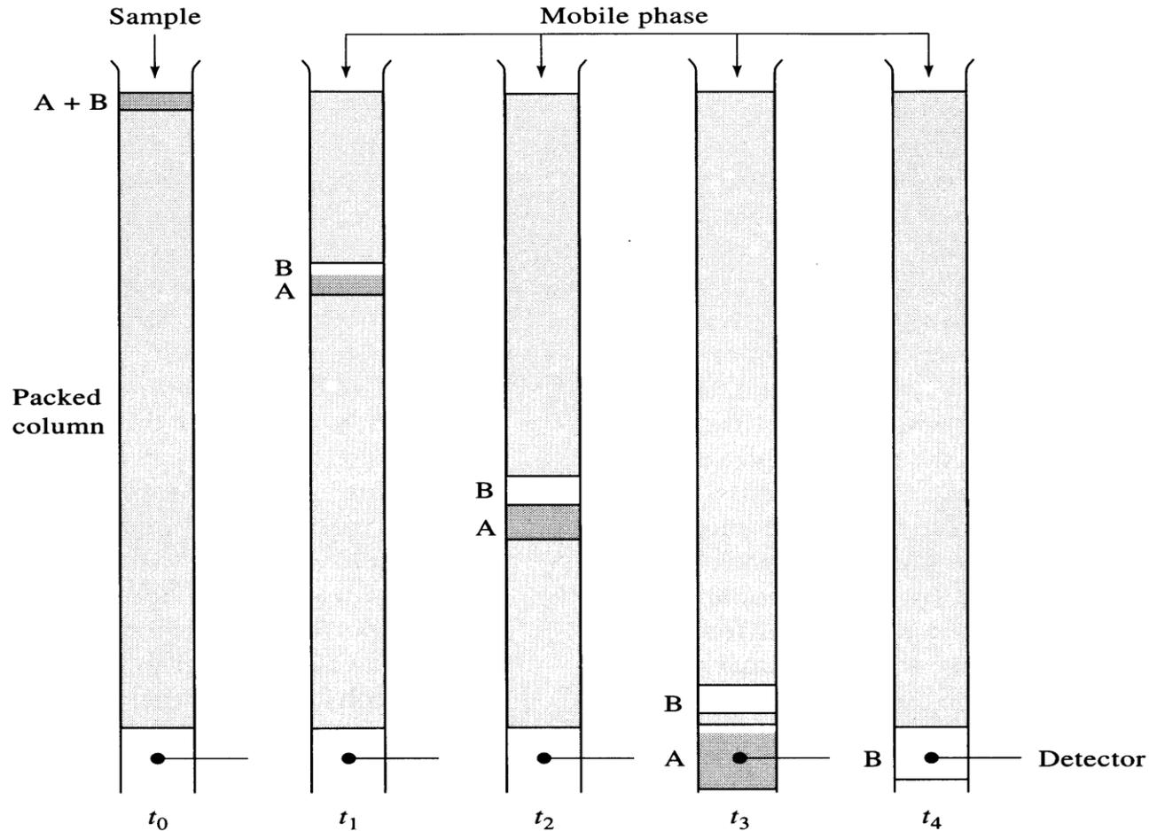
Fill the column with stationary phase. Then add mobile phase to remove air gas. Now put the mixture containing A and B on the top of the column. Now pass the mobile phase through column. Because of different adsorption capacity of solute molecule A and B will be distributed between stationary phase and mobile phase.
